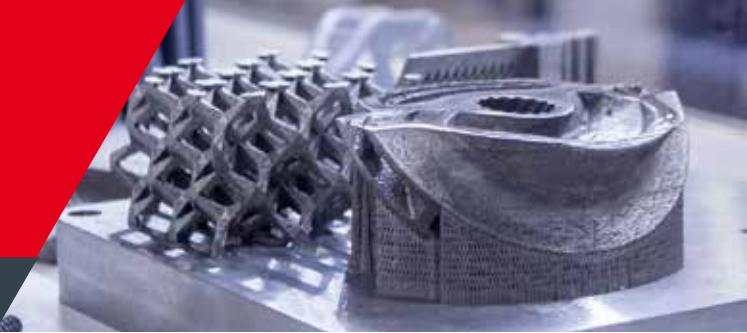
AMETEK Specialty Metal Products is committed to meeting the demands of Additive Manufacturing (AM) for mass-production of industrial components. We have engineered economic powders of mainstream stainless steel, nickel, and cobalt alloys for non-rotor-grade components made by Laser Powder Bed, Binder Jet, and Cold Spray processes.
