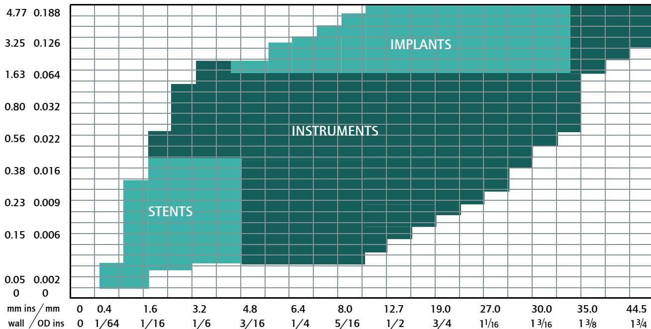
Size range for medical products is based upon manufacture of cold drawn tubing from 0.012 in (0.30 mm) to 1 5/8" (45 mm) OD. Tolerances: OD and ID up to 0.0005 in (0.0127 mm) are achievable.
