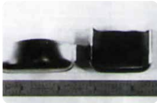
Figure 3. First Draw (left) and Fourth Draw (right) Battery Casing Part from AME205-899D Alloy.
